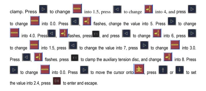
Note: when wrinkling value is greater than or equal to 3.0, the auxiliary tension disc must be set into clamped state. When wrinkling is none or less than 3.0, open the auxiliary tension disc. If left and right sleeves are to be sewn from the same starting point, press [52] to set into [11].
